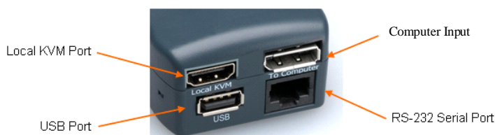
Figure 4-2 SpiderDuo Local KVM, USB, Computer Input and Serial Ports
