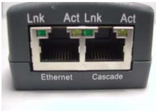
Figure 3-5 Spider RJ45 Ethernet and Cascade Ports
